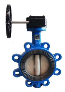
VESS is a resilient seated butterfly valve , with an EPDM / NBR rubber seat on valve body . The rubber sealing provides both sides bubble tight shut off and the pin design provides stronger and fixed connections between shaft and disc that ensure the stem stays firm during operation.
