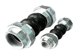
VESS Threaded Union Rubber Expansion Joint are designed for piping systems to absorb pipe movement, relieve stress, reduce system noise / vibration, compensate for misaligment / offset and to protect rotating mechanical equipment against start up surge forces. Compared to flange connected rubber joint, the threaded rubber joint are less weight and easier to install, special designed for threaded piping system. Twin sphere designs are more flexible and allow greater movement.
